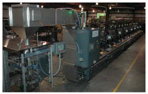
F-250 VFFS BAGGER, FAST AUTOMATIC WEIGHER (FAW), AND COUNTING TECHNOLOGY WITH ENHANCED DUAL VIEW SCANNING FROM BATCHING SYSTEMS, INC.
