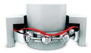
The SSB series is a popular choice among engineers, the single turn wave spring helps eliminate bearing play and minimize noise. The constant light/medium pressure they apply removes play between the ball bearings and the bearings' inner and outer races. Preloading can reduce the possibility of bearing damage due to vibration (vibratory loading) and wear due to repetitive and non-repetitive runout.
