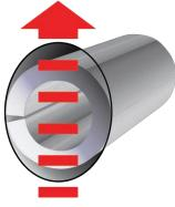
NON-DYNAMIC CONDITION INSTALLED SLOTTED PIN SHOWING THE "BUTTED" CONDITION MAKING THE PIN UNABLE TO ABSORB **DYNAMIC LOADS**
