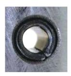
in hole damage (enlargement) and premature assembly failure.
