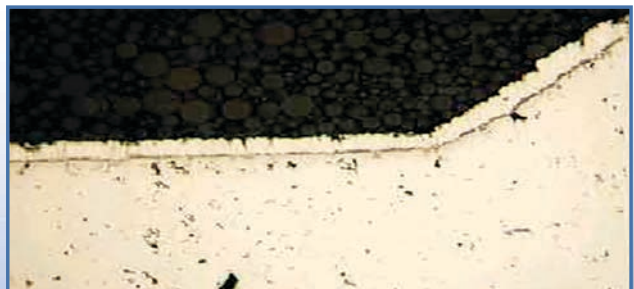
POWDER METAL PARTS AFTER ARMORGALV® (100 MICRONS/4MILS)
