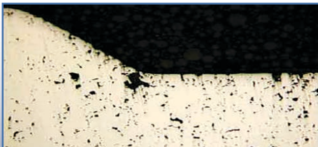
POWDER METAL PARTS BEFORE ARMORGALV®
