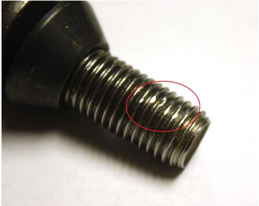
Fastener manufacturers must inspect each piece for small visual imperfections like burrs, scratches, thread damage or head cracks to dimensional measurement such as thread parameters, lengths, diameters, tapers, radii, straightness, perpendicularity, recess depth, and head protrusion.
